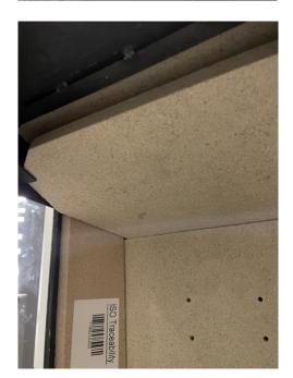
Lift Baffle in to place, Lift front section over brackets above each window and push up back until it rests over the rear brick. Make baffle rest inside side brackets
