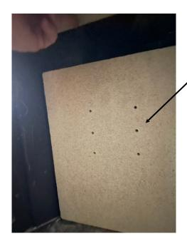
Whilst holding upper baffle in position place rear brick in place. Make sure holes in the brick are aligned with holes in rear of the stove.
