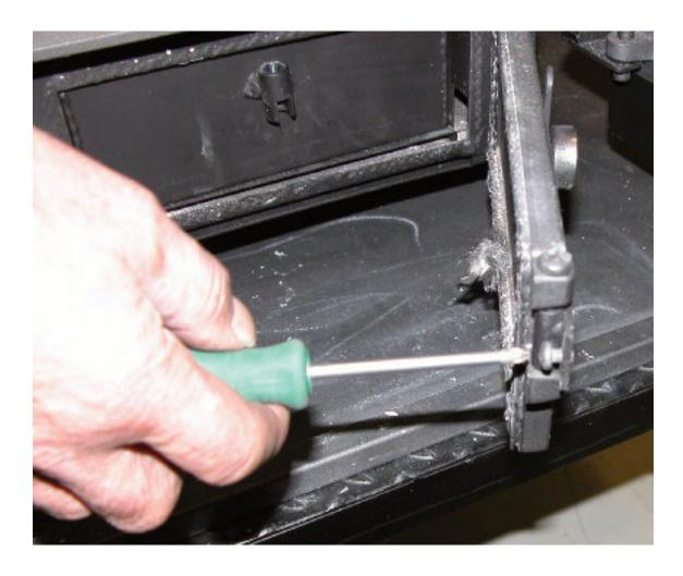
Adjust the screw at the end of the ash pan door lever to give a positive action when closing. Do not over adjust. The closing action of the lever should have a gentle resistance.
