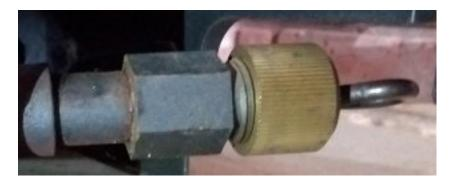
Every two weeks, if running a lot, or once a month, if not, undo the knurled nut half a turn, pull out the rod straight back then push it in turning it to clear any carbon out and this pushes it into the burner. This keeps the oil flowing well into the burner.
